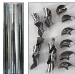
» Good surface finish due to stable chip formation and effective chip evacuation
