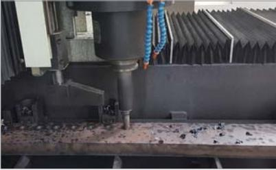
**Cutting condition**  $vc$  (m/min) = 47,  $fn$  (mm/rev) = 0.24,  $ap$  (mm) = 50, MQL (Mist)
