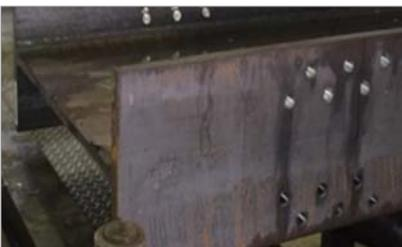
**Cutting condition**  $vc$  (m/min) = 56,  $fn$  (mm/rev) = 0.31,  $ap$  (mm) = 40, Wet
