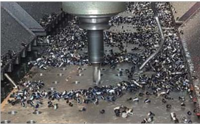
**Cutting condition**  $vc$  (m/min) = 80,  $fn$  (mm/rev) = 0.27,  $ap$  (mm) = 25, Wet
